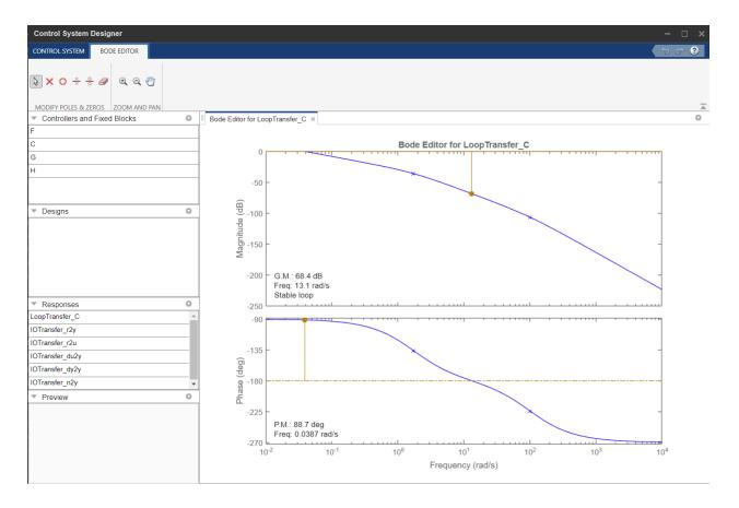
(a) Looking at the Bode plot, the gain margin is given as 68.4 dB
