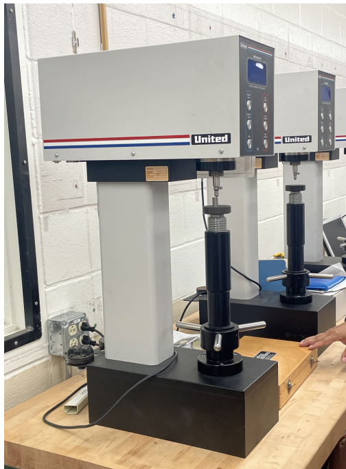
Figure 3: United Tru-Blue II Rockwell Hardness Testing System
