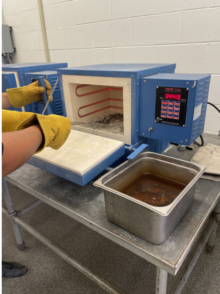
Figure 4: Paragon HT14D - Heat Treating Furnace
