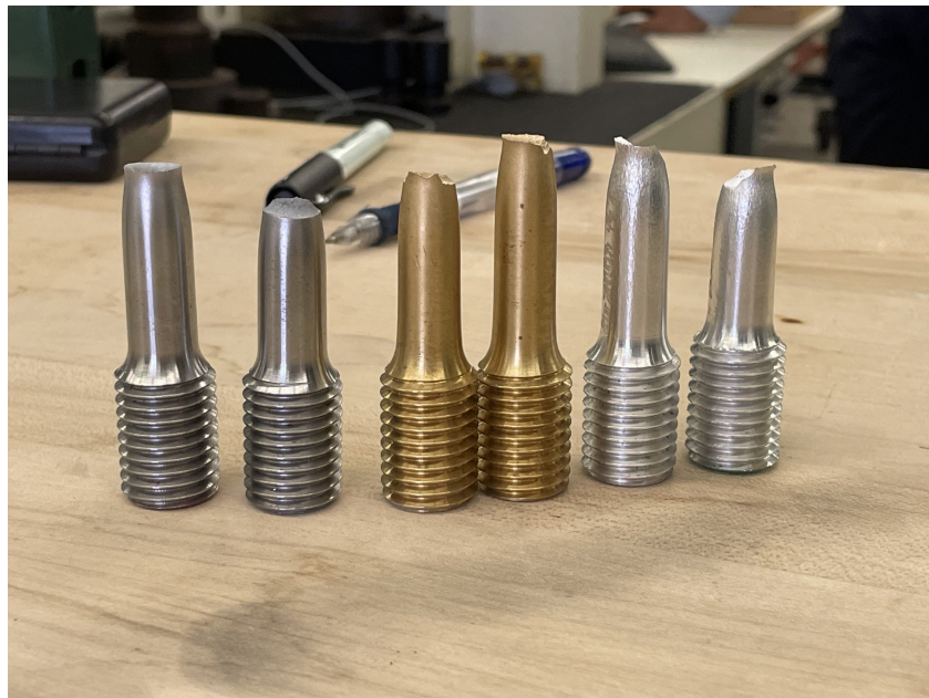
Figure 4: Fractured Steel, Brass, and Aluminum Specimen After Tensile Test (From Left to Right)
