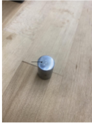
Figure 4. Image of The Material After Three Indentations On Its Surface
