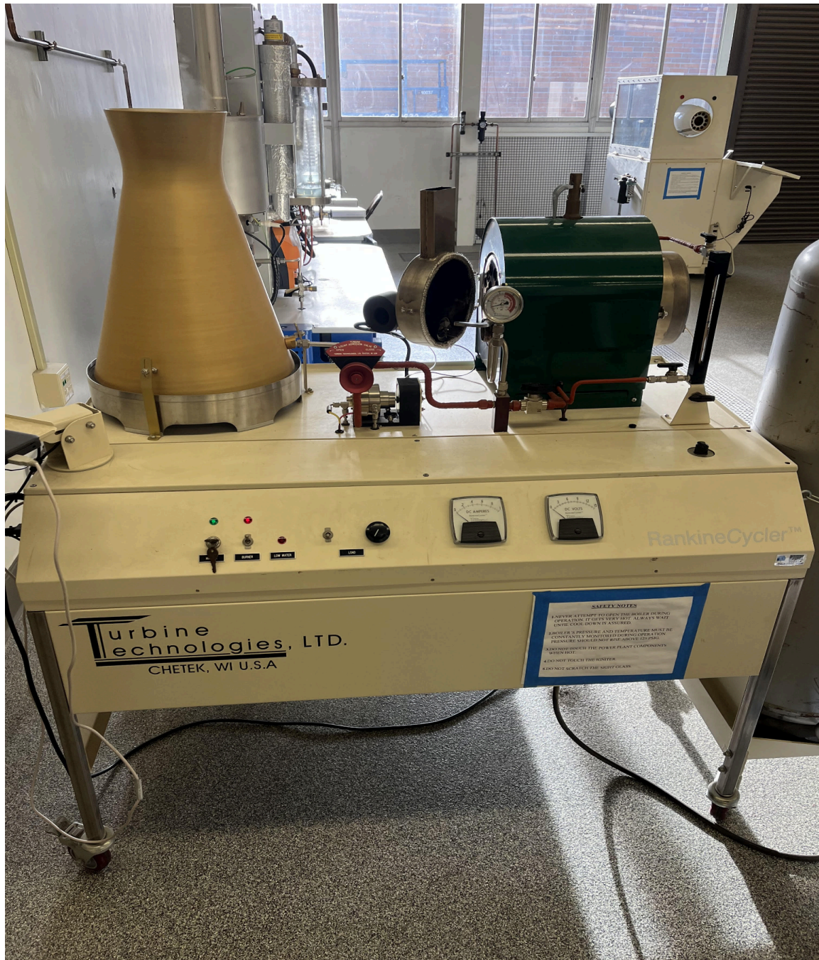
Figure 2: The Turbine Technologies Steam Power Plant.
